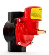
The mechanical earthquake valve that perceives the seismic activity (earthquakes), and automatically shuts off the flow of gas as a result of the perceived activities. This device has been designed to automatically shut off the gas flow due to earthquakes under TS12884 standard conditions. When the device is subjected to the momentum range of seismic vibrations given in the standard conditions, the device makes shut-off.
