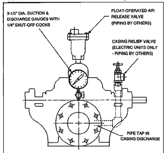
A casing pressure relief valve is provided for all electric motor driven Fire Pumps. It shall be installed in or piped to the tap in the side of the discharge neck on the pump casing. A separate outlet shall be piped to a drain to discharge the water from the relief valve.
