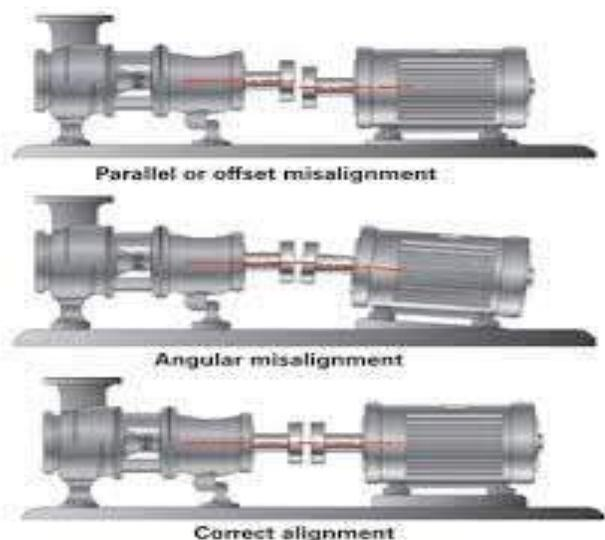
The faces of the coupling halves should be spaced far enough so that they do not strike each other when the driver coupling half is moved hard over toward the pump and due allowance shall be provided for wear of the thrust bearings.
